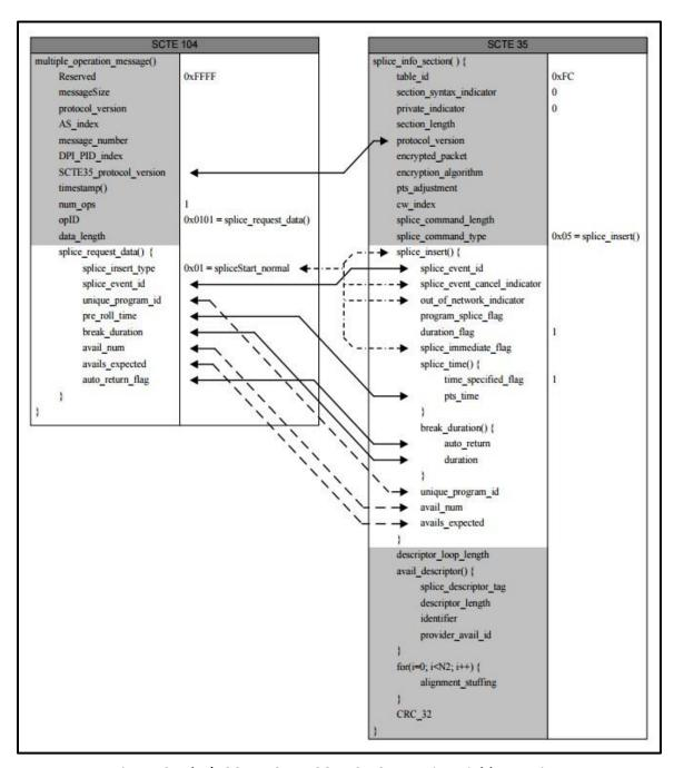
Figure 2: Alta's SCTE-104 to SCTE-35 Conversion Field Mapping
