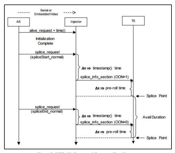
Figure 3: SCTE-104 Command One-way Flow Diagram
