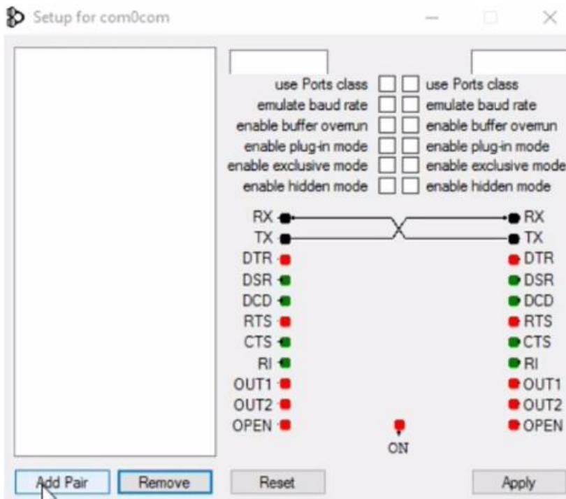
2. Highlight the *Virtual Port Pair*, then select *use Ports class*, *emulate baud rate*, and *enable buffer overrun* in both columns.
